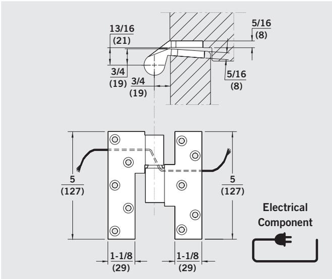
**No. 75200** — Electrified intermediate pivot for power transfer. Available as an eight-wire design using #28 AWG, rated for 24 V maximum. Pairs of wires connected together provide 2 A maximum. Multiple pairs provide greater amperage ratings, i.e. two pairs in a circuit provide 4 A maximum and four pairs provide 8 A maximum. Pivot is non-load bearing and has non-separable pivot leaves.
