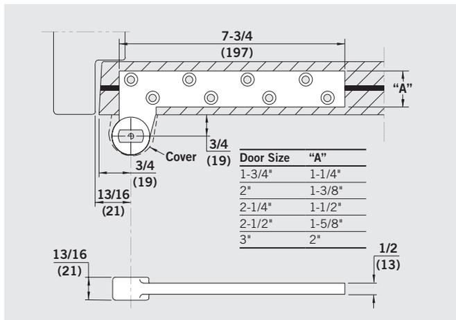
**No. 75343** — 3/4" offset standard steel bottom arm for lead-lined 1-3/4" doors. Can also be used on fire doors rated up to 3 hours. For use with 7471K and 7471HD floor bearing.
