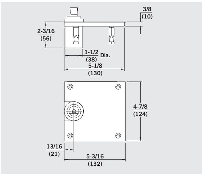
**No. 7471HD** — Heavy-duty floor bearing for center hung doors weighing up to 1000 lb and offset hung doors weighing up to 800 lb. Can also be used on fire doors rated up to 3 hours. For use with No. 7421, 75323, 75343 and 15323 bottom arms. Interchangeable spindles provide for bottom door clearances of 3/8" to 1-3/4". Includes cover plate. Bearing is mortised into floor. Interchangeable spindles and associated bottom door clearances shown in the adjacent chart.
