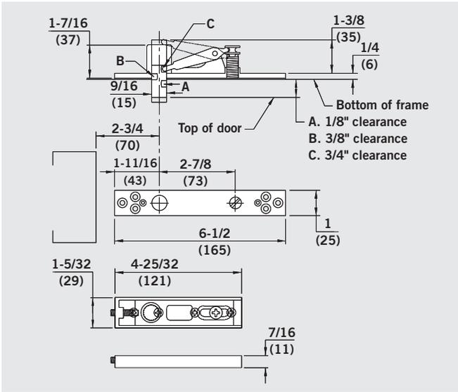
**No. 8062** — Walking beam top pivot with cover plate. Lateral adjustment assures the door is plumb. Accommodates top door clearances of 1/8", 3/8", or 3/4". Optional extended pin available for clearances of 3/4", 1", or 1-5/16". Not recommended for use with overhead stops/holders. Use HD8062.
