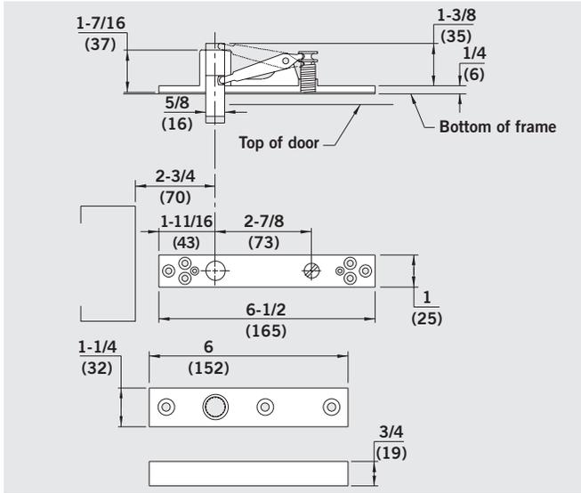
**HD8062** — Heavy-duty walking beam top pivot with frame portion and cover plate. Door portion consists of a needle bearing pressed into a 3/4" thick aluminum block. Adjustable to obtain a 1/8"-3/8" clearance between the door and frame. Required when using overhead stops/holders.
