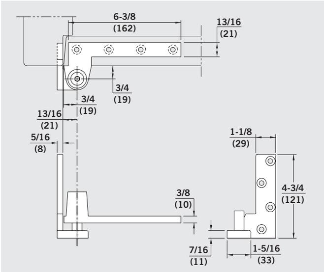
**No. 75320** — 3/4" offset brass bottom side jamb pivot. For use with doors weighing up to 350 lb. Has a vertical height adjustment of 3/8".
