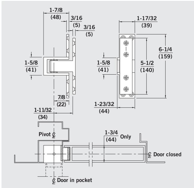
For use on doors up to 4'-0" wide and weighing up to 300 lb when hung on three pocket pivots. Allows for maximum door swing of 90°
