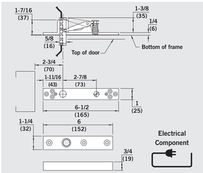
**E8062** — Electrified walking beam top pivot for power transfer. Available in a two wire and four wire design using #18 AWG. Both designs provide a maximum of 6 A at 24 V. Specify number of wires required.
