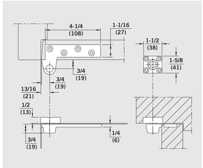
**No. 75120/102** — Standard mortised door portion with a pivot block containing a needle bearing mortised into the overhead condition above. This pivot is ideal for conditions when the door is inset from the frame face, or the ceiling is directly above the door.
