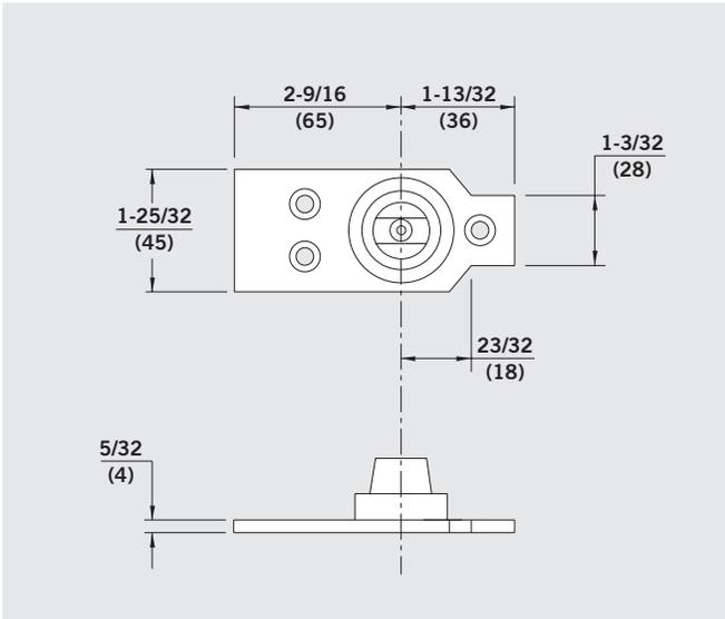
**No. 7471K** — Standard floor bearing with thrust roller bearing for doors weighing up to 440 lb. Can also be used on fire doors rated up to 3 hours. Includes cover cap. Mounts directly to floor. For use with No. 75323, 75343, 7421, 7422 and 15323 bottom arms. Available with integral spindle extensions as shown in the adjacent chart.
