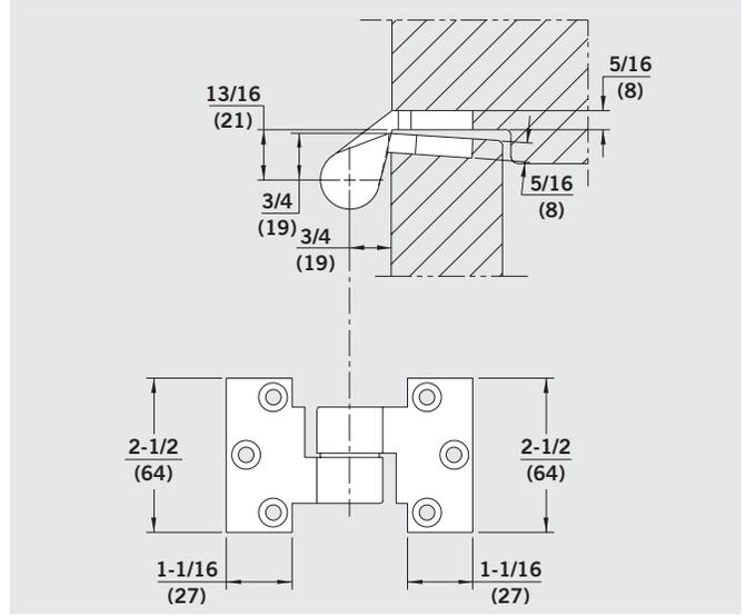
**No. 75210** — 3/4" offset light-duty brass intermediate pivot. Non-load bearing, for door alignment only.
