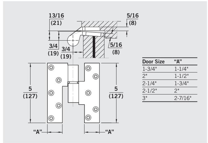
**No. 75240** — 3/4" offset brass intermediate pivot for lead-lined doors 1-3/4" thick.
