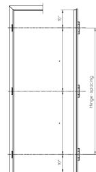
The hinge spacing does not increase the load capacity! Note: We recommend for all exterior doors the use of three hinges.
