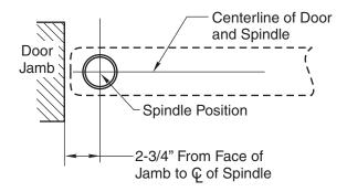
A. Measure 2-3/4" out from door jamb on centerline of door. This is the location of the spindle center.
