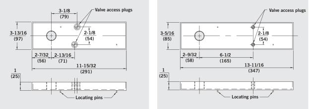
Made from stainless steel and used in lieu of standard floor plate. Offers uninterrupted appearance with terrazzo or marble. Shims are included to allow easy removal of pan after initial installation.
